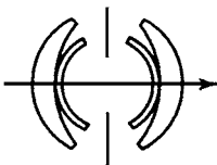
Figure 17.12 The Topogon lens (U.S. Patent 2,031,792-1936) covers 90^\circ to 100^\circ at a speed of f/8 .
